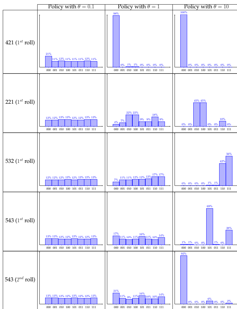
FIGURE 9.3: Mixed (randomized) policy provided by the soft value iteration (SVI, Equations (9.39)-(9.40)), for some interesting cases. The resulting policies interpolate between a uniform distribution (equal to the reference transition probabilities, left) when \theta \rightarrow 0 and the deterministic, optimal, policy obtained by the value iteration algorithm (sum of Kronecker delta, right), when \theta \rightarrow \infty .
